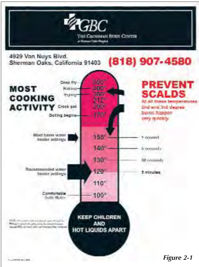
Figure 2-1. Length of time required for second- and third-degree burns to occur when exposed to liquids of varying temperatures, reinforcing the relative importance of time and surface temperature in the causation of cutaneous burns.
